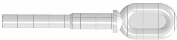
Figure 3. Cutting the workpiece with a finite number of parallel planes perpendicular to its longitudinal direction
