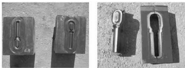
Figure 11. Forging die and cutting die used for forging electric tension rod
